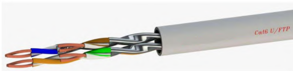
LAN cable with 4 pairs, category 6, with individual Al-foil screen
